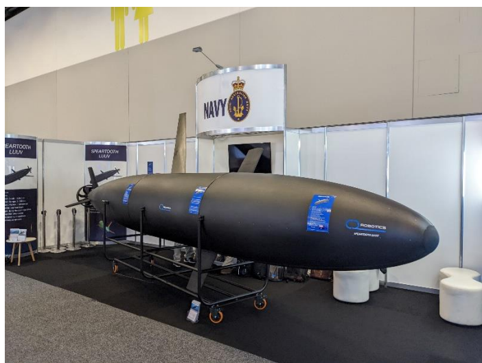
Figure 4.4: C2 Robotics' Speartooth large uncrewed underwater vehicle
