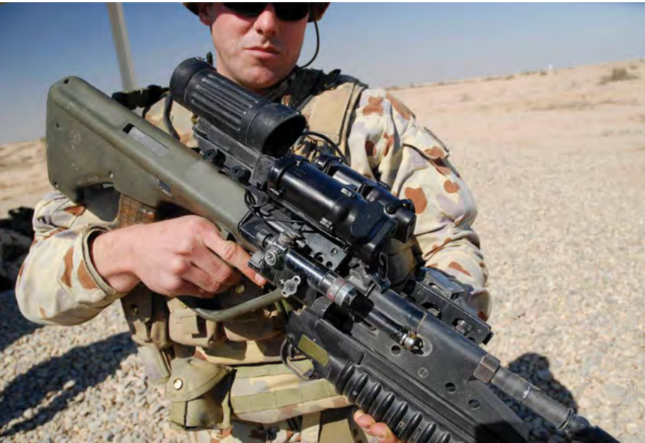
An Australian soldier in Iraq holds an F88 Steyr assault rifle fitted with an assortment of equipment, including the new laser attention gaining device. Below that is a night aiming device, and to the rear is an optical sight. Beneath the barrel of the weapon is a grenade launcher attachment. Photo: Australian Department of Defence, online .
